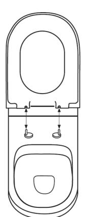
To fit seat, slide seat down onto stainless steel pins.
